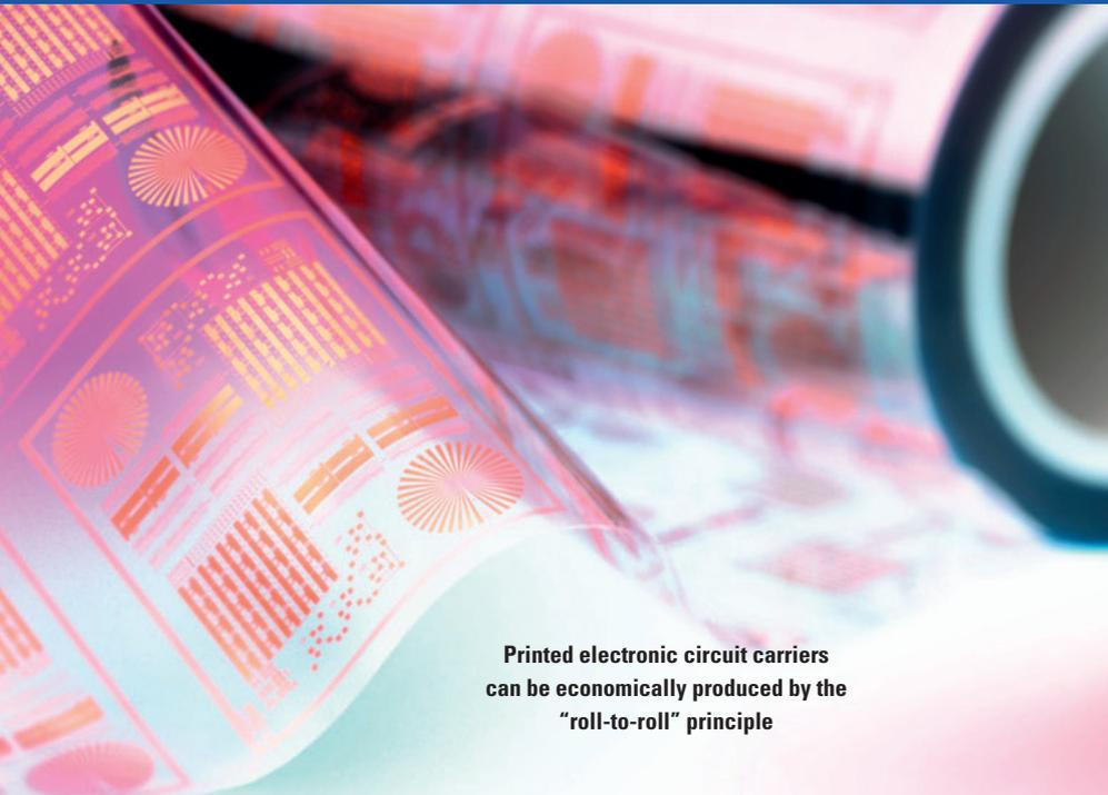
Printed electronic circuit carriers can be economically produced by the "roll-to-roll" principle
