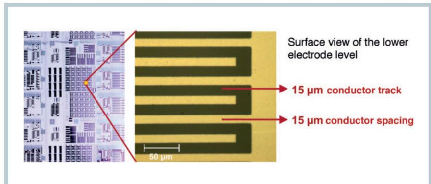
**Fig. 2. Results of the PolyIC production process: high-resolution structures on a flexible substrate**
