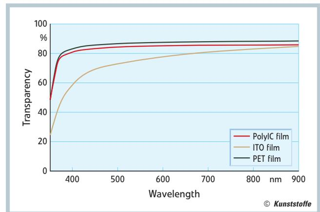
Fig. 5. Transparency of the PolyIC conductive coating as compared with ITO films
