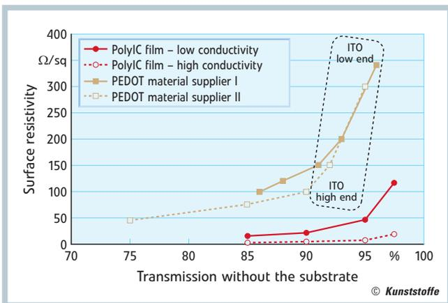
Fig. 4. PolyIC technology: transparency and conductivity as compared with alternative materials
