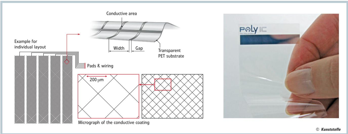
Fig. 3. Layout pattern for a transparent, conductive coating: details of an individual layout (left), pattern (right)
